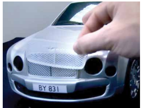
Bentley Motors designers print miniature scale models of vehicle interiors and exteriors.
