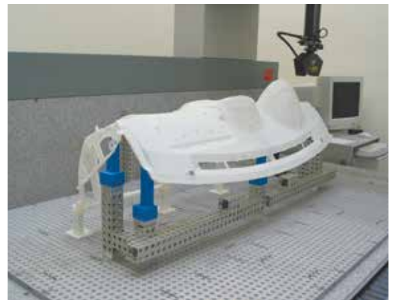
Hyundai Mobis 3D printed an instrument panel in ABS plastic to measure component fit.
