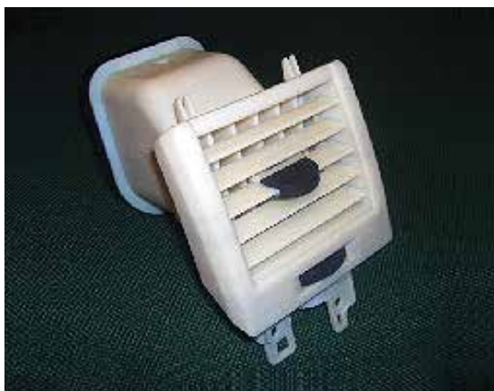
Jaguar Land Rover used The Objet500 Connex 3D Printer to print a complete fascia air vent.
