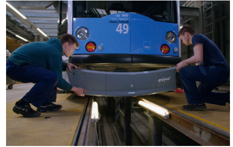
Installation of the 3D printed housing cover
