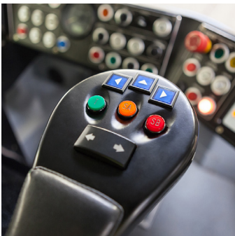
3D printed armrest with three extra buttons for the control system.
