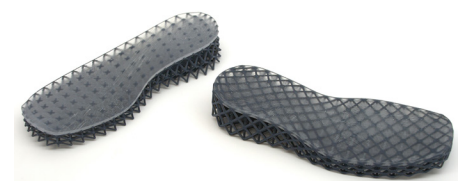
DManD researchers created multi-material soft-lattice structures for this footwear prototype using a custom slicer to control stiffness and behavior of the material.
