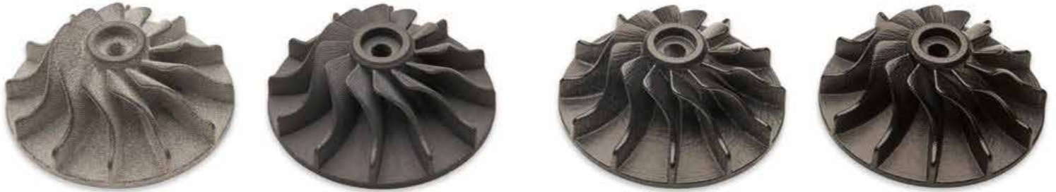
Finishes left to right: Unfinished part, media blasting, dyed, tumbled and vibratory finished
