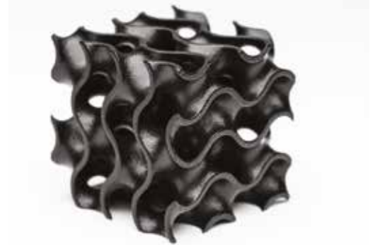
This gyroid has been chemically smoothed and dyed.
