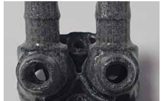
Tubes allow for easier powder removal.
