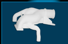
SLS Complex ducting
