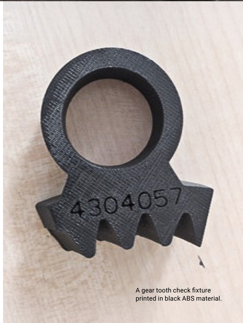
This gear teeth check tool was printed with ABS thermoplastic.
