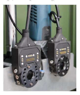
It is vital that the connector can be utilized on various tools and withstand high currents. Each high current power pin can take up to ten amps. The lower current data pins are able to reliably pass an amp each.
