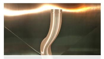
A duct built in a vertical orientation to improve sealing and surface finish.
