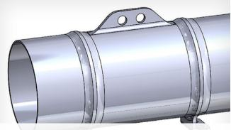
FDM ECS ducts with integral mounting flanges can be produced as a single-part design.
