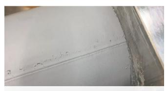
Standard automotive or aerospace paint can be used as a sealant for low-pressure applications.
