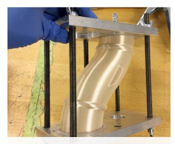
An S-shaped duct used for remnant fill testing.
