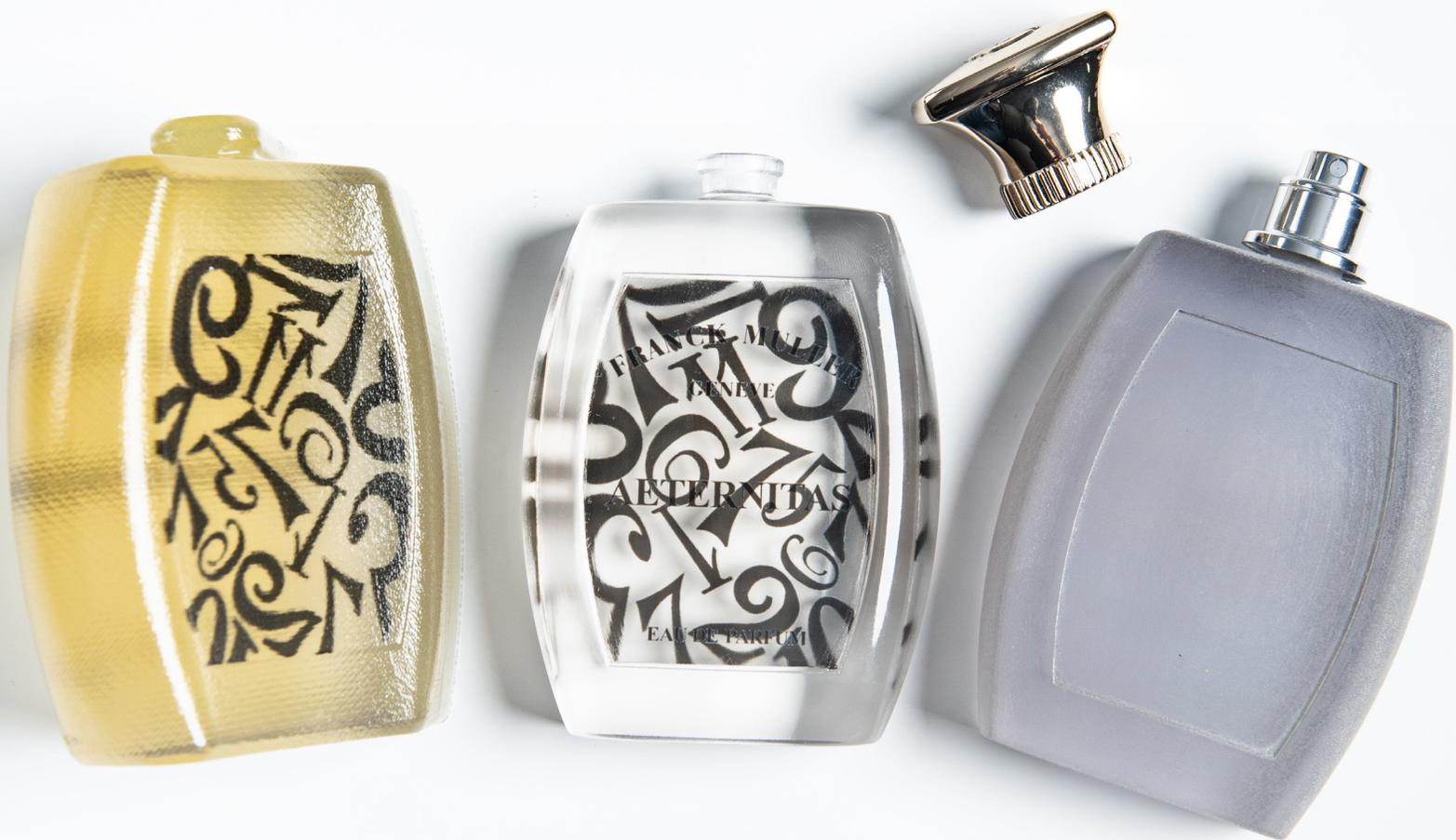
The left sample is an unfinished bottle. The right sample was produced with an older version of clear and the middle one has been produced and polished with Stratasys' new clear material.
