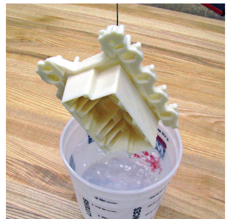
Figure 5: Dip components (shown) in solvent, or apply it with a brush.
