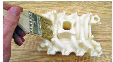
Figure 8: Apply epoxy adhesive and brush over surfaces.
