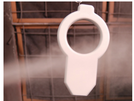
Figure 4: Apply paint to seal surface.
