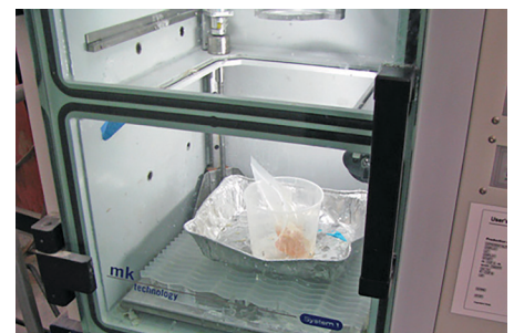
Figure 11: Draw a light vacuum to pull epoxy into the part.
