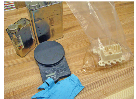
Figure 9: Manifold (right) immersed in two-part epoxy.
