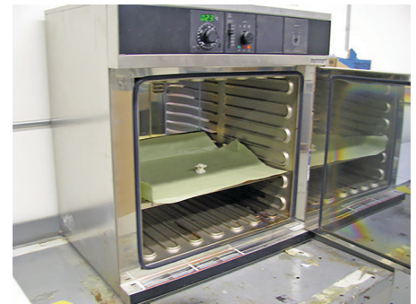
Figure 10: Condition part and epoxy in an oven.
