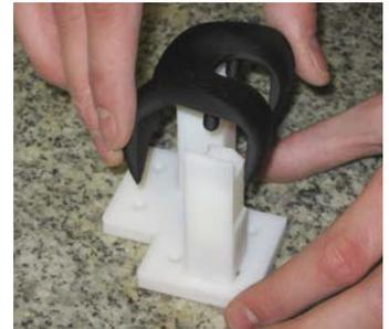
Figure 2: FDM contact elements designed to support an artificial knee.
