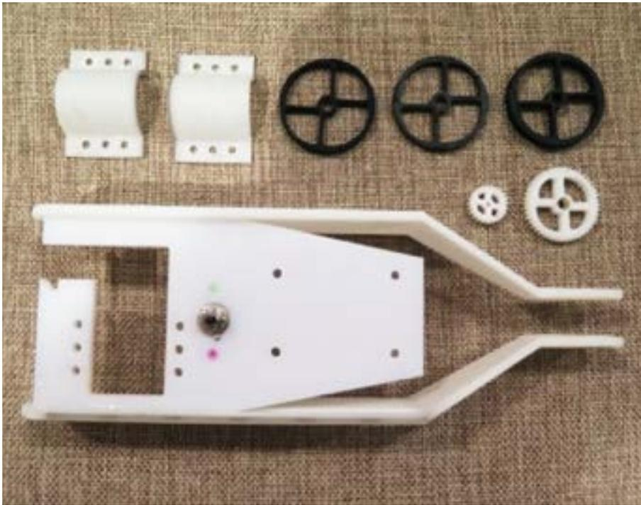
3D printed solar car components before assembly.
