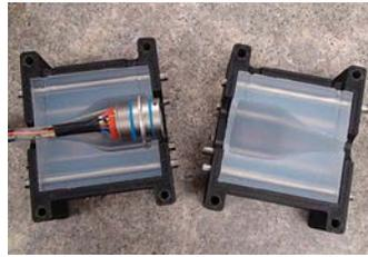
RTV silicone mold for overmolding operation
