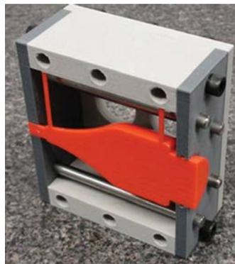
Silicon mold box with alignment pins
