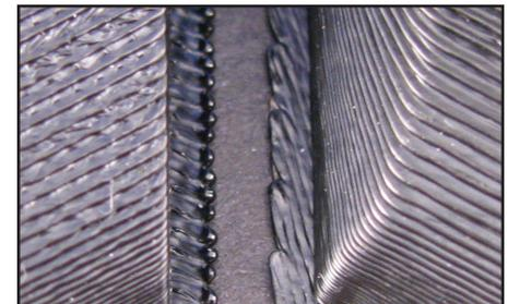
Figure 57: On shallow slopes, raster turnarounds may be visible (left). Custom groups can correct this (right).
