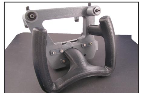
Figure 10: Redesigned FDM tool consolidates most components (ABS-M30).
