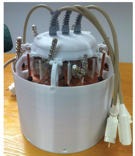
Figure 3: MRI head coil required compatible materials (PC-ISO).
