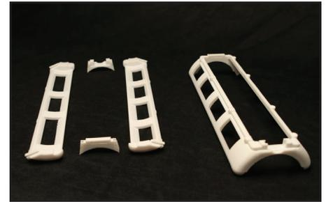
Figure 8: Part split into pieces to aid in assembly of final product (polycarbonate).
