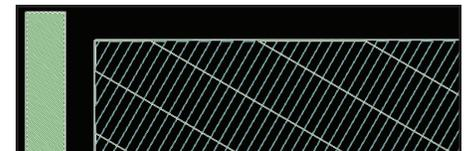
Figure 76: Wide supports in Custom Group 1 run perpendicular to default supports.
