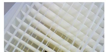
Figure 69: Top-down view shows wide spacing between support rasters.
