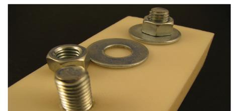
Figure 15: Fasteners may be mounted to FDM parts (ABS-M30).
