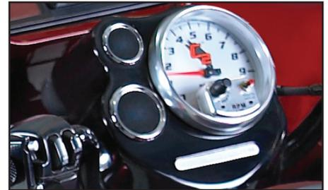
Figure 5: Gauge pod for custom motorcycle (painted polycarbonate).
