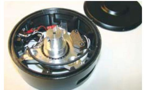
Figure 2: Electronic surveillance equipment includes FDM housing (ABS-M30).
