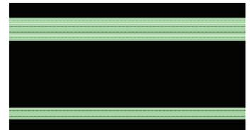
Figure 19: CAD revisions produce a constant wall thickness that has a solid, dense fill.
