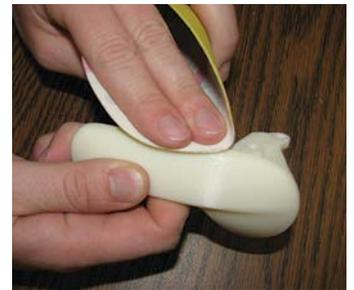
Figure 1: Hand sanding is one option for part finishing, but it may be prohibitive due to cost and time.
