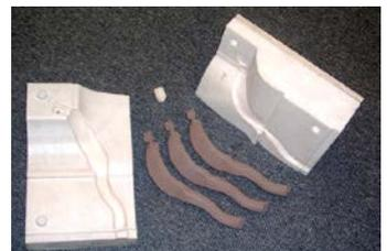
Figure 7: Sand casting cores (center) are made from FDM core boxes (left, top center, right) with smooth surface finishes.
