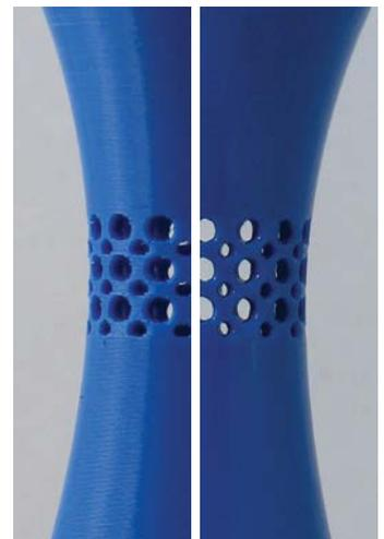
Figure 3: An FDM part (left), after removal from the Smoothing Station (right)
