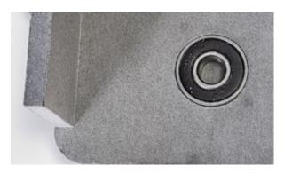
Press fit bearing seat printed directly into the part for a lead screw. For bearings to be fit, these require a high level of accuracy delivered by SAF™ PA12.
