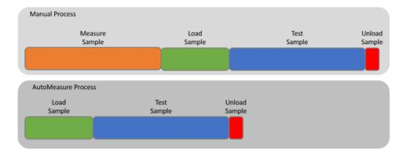
An additional benefit of the AutoMeasure is an improvement in repreatability of measurements. Removing the variation of different operators removes the chances for differences in technique influencing measurement results.
