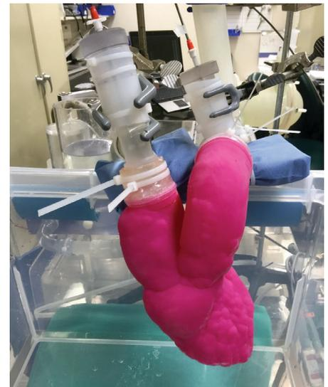
Aortic stenosis flow testing performed on a patient-specific 3D model.
