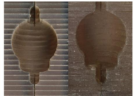
3D printed sectioning block used for rodent brain dissection. The slices created by the segmentation fixture are 2 mm thick and the slots allow a 200 micron blade.
