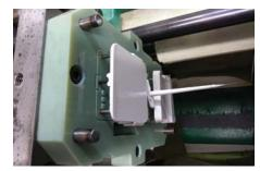
Injection molded part being ejected from 3D printed mold.
