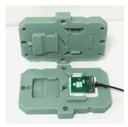
3D printed injection molds created in Digita ABS material.
