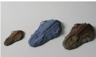
SCEC, a Korean manufacturer of exhibition models, won an aquarium project with its 3D printing capabilities. 3D printed models of aquatic life, (center) appear lifelike after post-processing (left and right).
