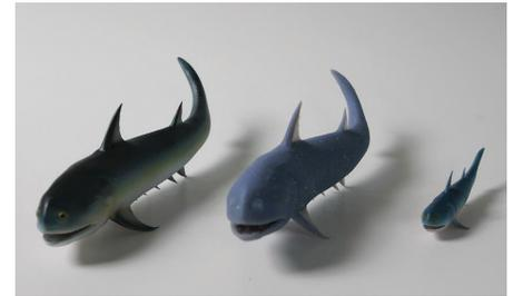
These 3D printed replicas of a shark show a version right off the printer (center) and post-processed (left and right) for detailed teeth and sharp fins.
