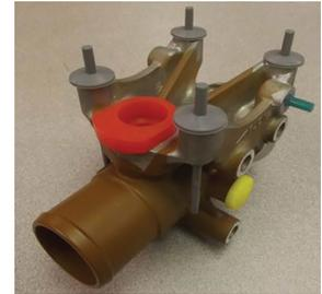
After the 3D printed design is verified, final masks can be production molded.
