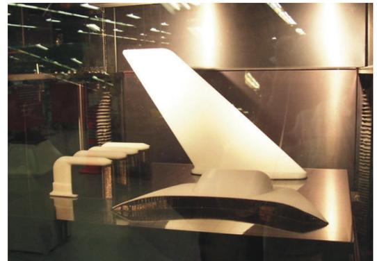
UAV replica fuselage and wings, manufactured with the FDM process.
