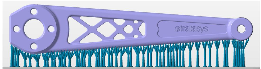
Once iteration is completed the vertical and support-free orientation would be preferred.
