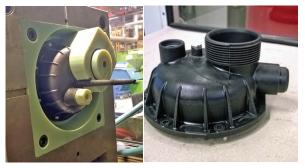
Mold inserts (left) and the final injection-molded part (right).
