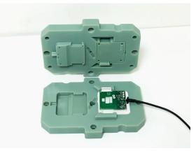
A 3D printed mold created in Digital ABS material by Arad Group.
