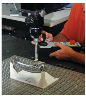
Using AM fixtures, Oreck completes CMM programming before first
