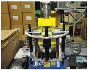
At Thogus / rp+m, production aids, such as the vellow safety shield and gray diverter (foreground), have proliferated with additive manufacturing.
