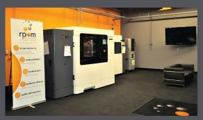
Three of rp+m's FDM additive manufacturing machines
