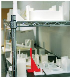
Additive Manufacturing made fixtures are prevalent in Oreck's QA lab.
