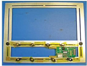
Machined carrier with manually applied tape for masking.
