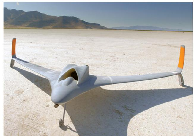
Final 3D printed jet-powered aircraft.
