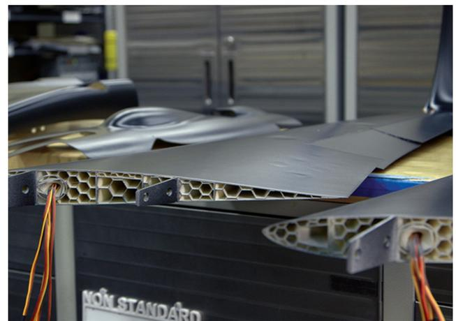
Internal wing design, optimizing complex internal structures, for lightweighting aircraft.
