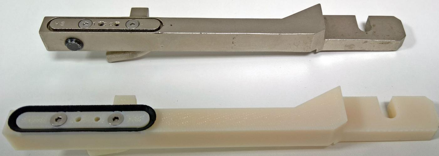
UPSA is making 95% cost-savings on just one part alone by replacing cast steel arms with high-performance 3D printed arms using ABS-M30i 3D printing material.
