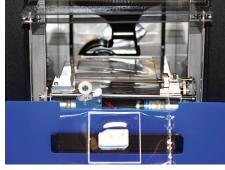
A part produced with the Continuous Build Demonstrator being ejected into the catch bin
