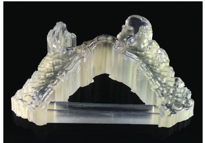
A complete model, like this frame with the support material intact, takes only 65 minutes via the digital method, compared to two days with traditional methods.
