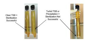
Figure 3: Determining success of sterilization procedure
