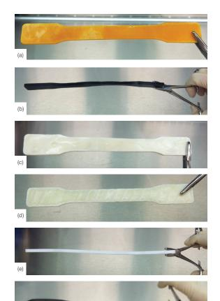
Figure 6: Material changes caused by flash autoclave, (a) ABSi: bending and color change, (b) ABS-ESD7: bending, (c) ABS-M30: bending and indentations, (d) ABS-M30i: bending and indentations, (e) PC: bending, (f) PC-ABS: bending
