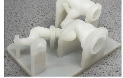
The final part after post processing and clean up. The flexible support structure allows the anatomical model to move whilst still being held in place.
