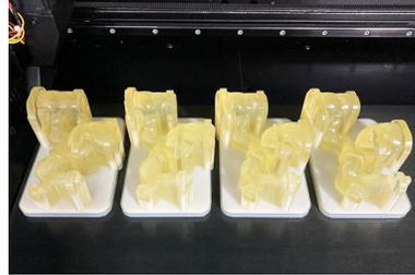
A series of designs of vessel models related to the liver, that was printed on the J750 Digital Anatomy Printer varying material properties and design features
