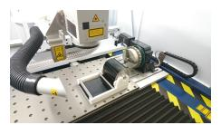
Kratzer now 3D prints fixtures for their laser devices, allowing the company to engrave multiple parts simultaneously, resulting a 90% time savings compared to traditional manufacturing.
