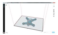
GrabCAD Print allows designers to convert CAD files and send to printer.
