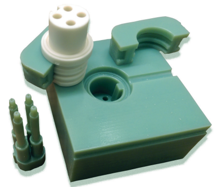
Complex component molded in a 3D printed mold
