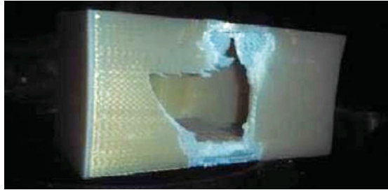
Figure 12 Real life test showed a part failure at 17 kg loading. The location of the stress concentration was the same as in simulation.
