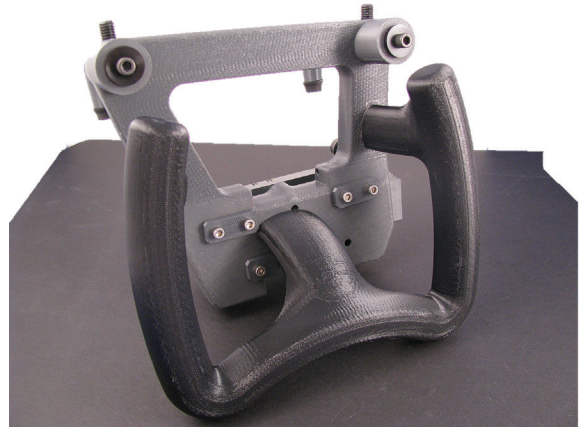
This redesigned FDM tool consolidates most components.
