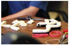
In his workshop in Nemours' pediatric engineering research lab, Whitney Sample has developed and 3D printed custom WREX devices for 15 of his smallest patients. Resistance bands relieve the force of gravity on the arms, much like the springs on a swing-arm lamp keep it suspended in air.
