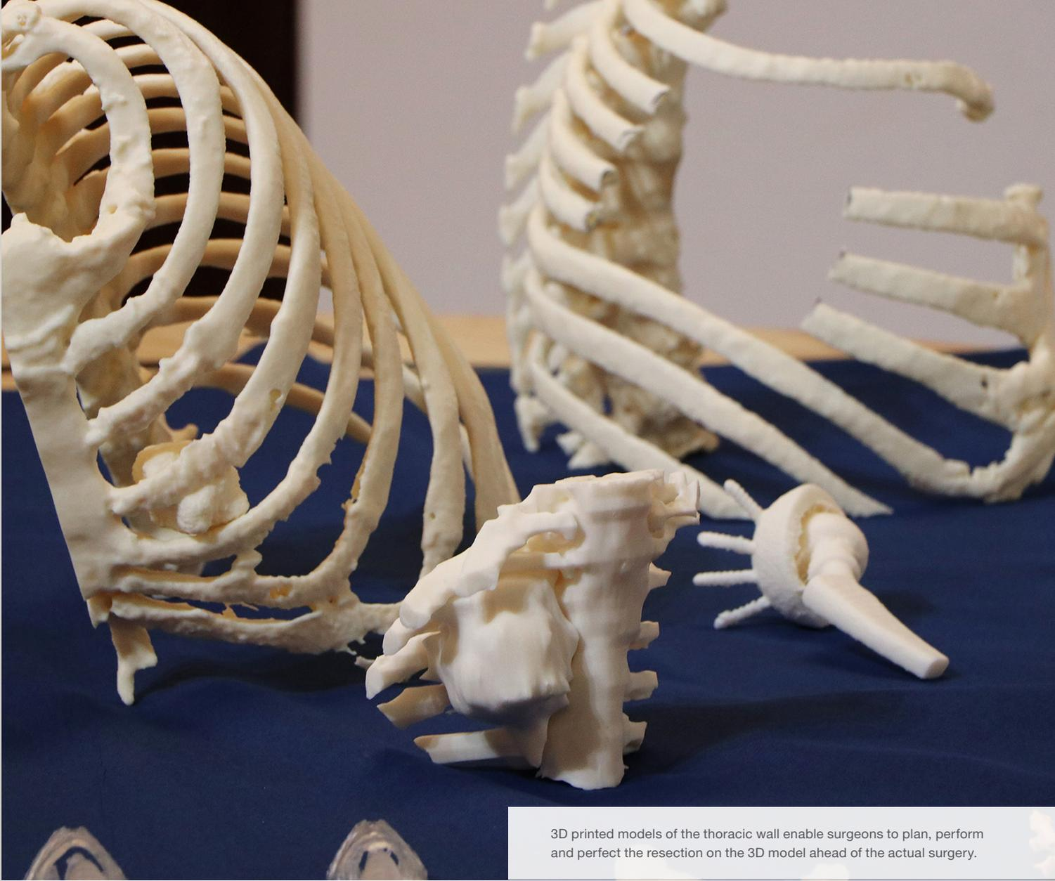
3D printed models of the thoracic wall enable surgeons to plan, perform and perfect the resection on the 3D model ahead of the actual surgery.
