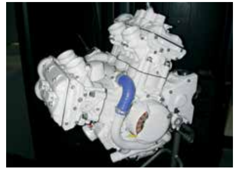
The Desmosedici's engine was prototyped almost entirely from polycarbonate using the FDM process.
