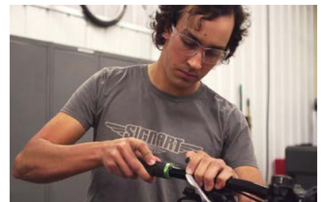
Trek engineering tech Patrick Zeigle mounts a multi-material 3D printed grip onto a bike for testing.
