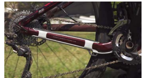
Trek's Objet500 Connex3 created this durable Digital ABS chain guard with rubber-like components in one print job.
