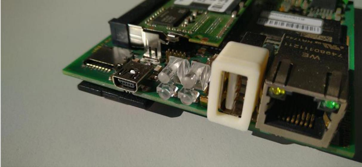
3D printed prototype of a USB port
