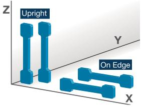
Figure 1: Test sample orientations
