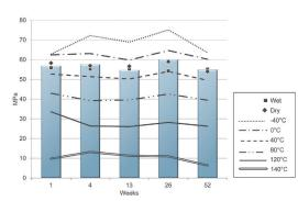
Figure 2a: Tensile strength - 20 °C, controlled environment, on edge.
