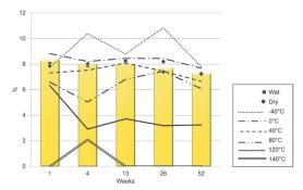
Figure 4a: Elongation at break - 20  $^\circ \rm C,$  controlled environment, on edge.
