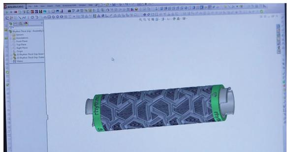
CAD model of an overmolded handlebar grip
