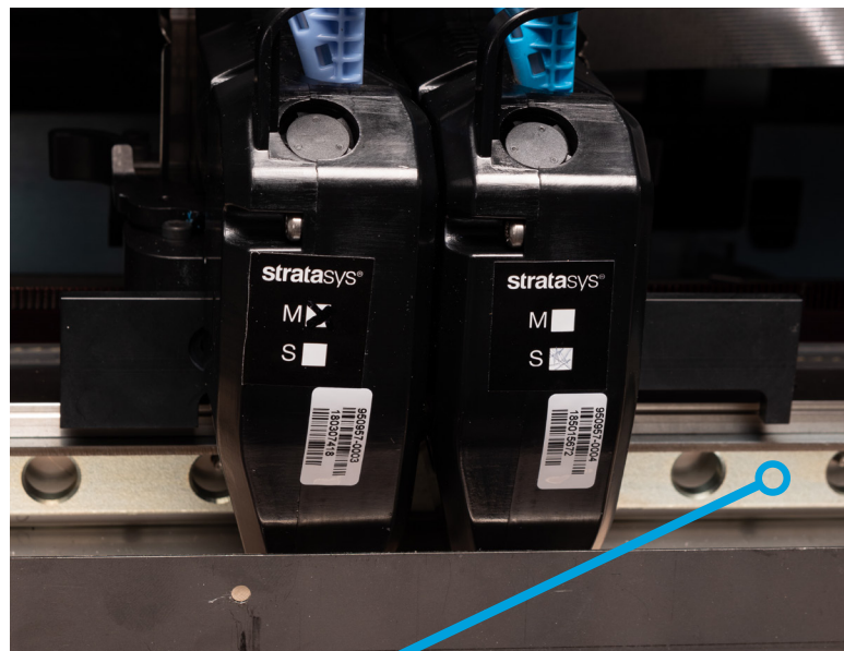
Head rail I-beam reinforcement
