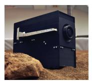
TransRoPorter Prototype with FDM 3D printed components.
