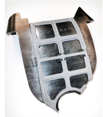
3D printed emblem locating fixture with carbon fiber frame (gray) and TPU backing.
