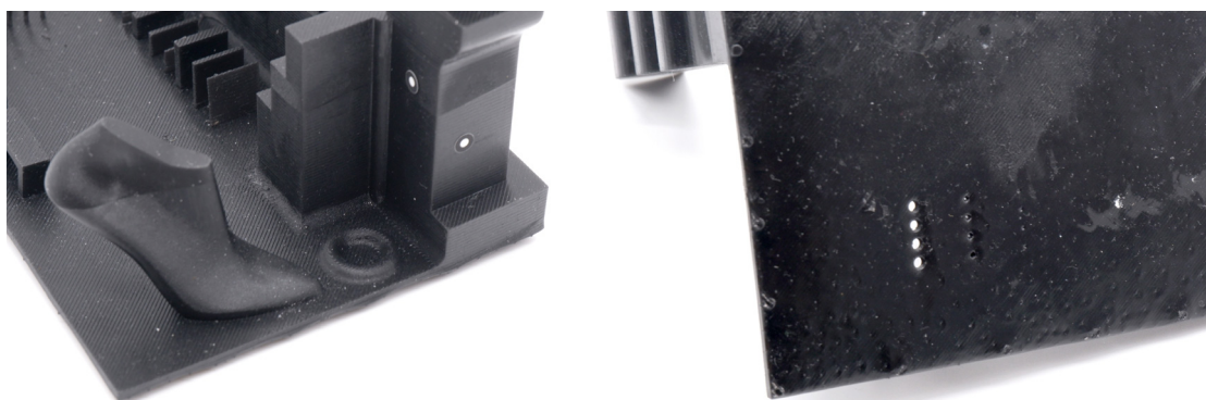
Surface defects and muddy features resulting in unreadable text
