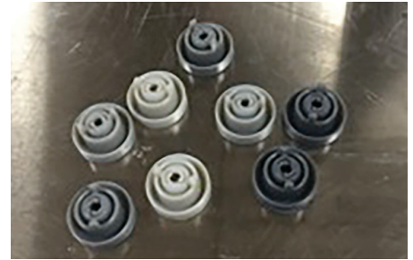
Multi-material Roomba prototype parts 3D printed with PolyJet technology.
