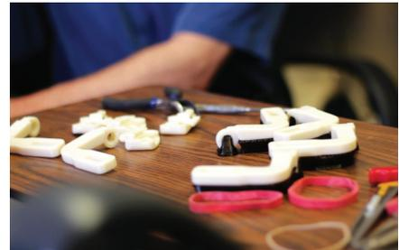
In his workshop in Nemours’ pediatric engineering research lab, Whitney Sample has developed and 3D printed custom WREX devices for 15 of his smallest patients. Resistance bands relieve the force of gravity on the arms, much like the springs on a swing-arm lamp keep it suspended in air.
