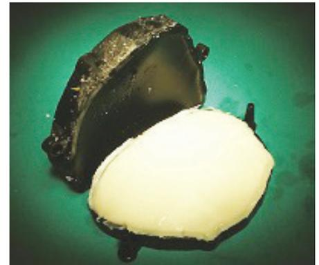
3D printed mold with bone prosthetic.
